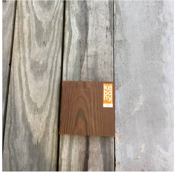
New Kebony lying on 3-year-old Kebony decking alongside 20-year-old gunite (concrete) pool edge
